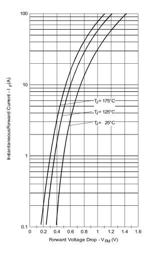
Fig. 1 - Maximum Forward Voltage Drop Characteristics
