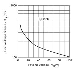
Fig. 3 - Typical Junction Capacitance vs. Reverse Voltage
