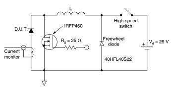
Fig. 8 - Unclamped Inductive Test Circuit
