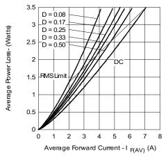
Fig. 6 - Forward Power Loss Characteristics
